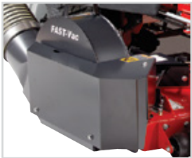
Extra wide 7" diameter outlet hose
